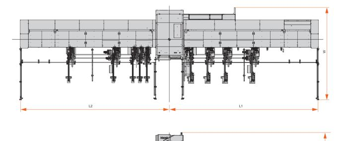
Shown with 8 m loading and unloading unit and optional chain conveyor. Chiller unit, transformer and optional dust collector not included.
