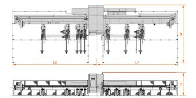
Shown with 8 m loading and unloading unit and optional chain conveyor. Chiller unit, transformer and optional dust collector not included.
