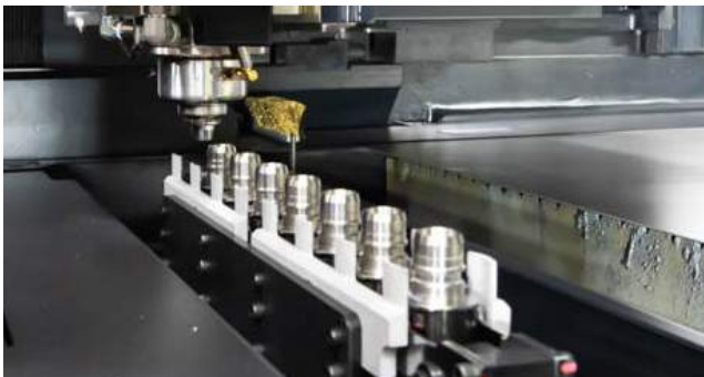
Auto Nozzle Changing reduces operator errors, improves consistency of operation and lowers operator dependency.
