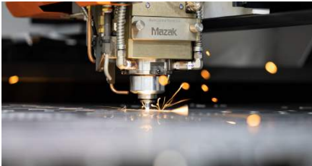
Pierce Detection senses when the pierce breaks through the material as compared to a programmed pierce that would include added time to account for variations in the process.
