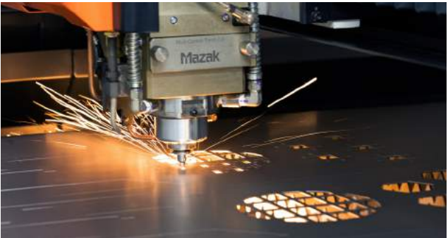
Flash Cut strategies synchronize turning the laser ON / OFF with axis movement to increase throughput.
