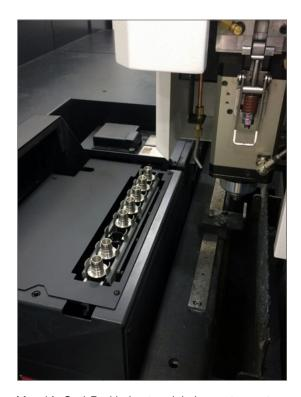
Mazak's Opti-Pod helps to minimize system setup time and improve extended unattended operation while maintaining optimized machining conditions.
