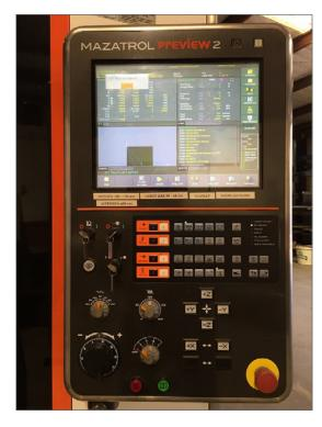
Mazak's PreView II control has a 15" touchscreen and its straightforward user interface helps to simplify machine operation.
