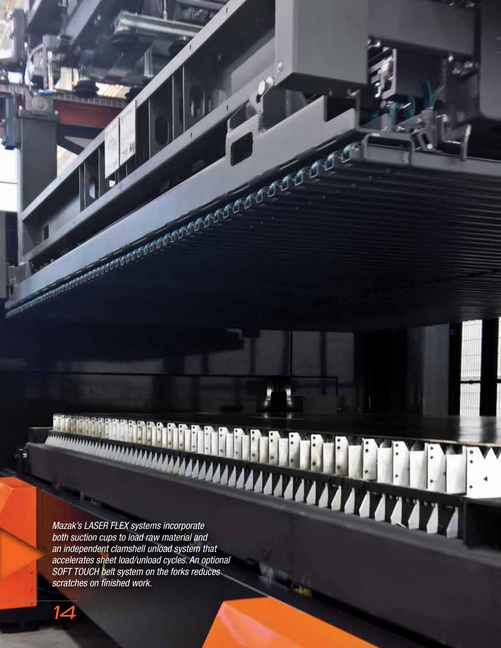
*Mazak's LASER FLEX systems incorporate both suction cups to load raw material and an independent clamshell unload system that accelerates sheet load/unload cycles. An optional SOFT TOUCH belt system on the forks reduces scratches on finished work.*
