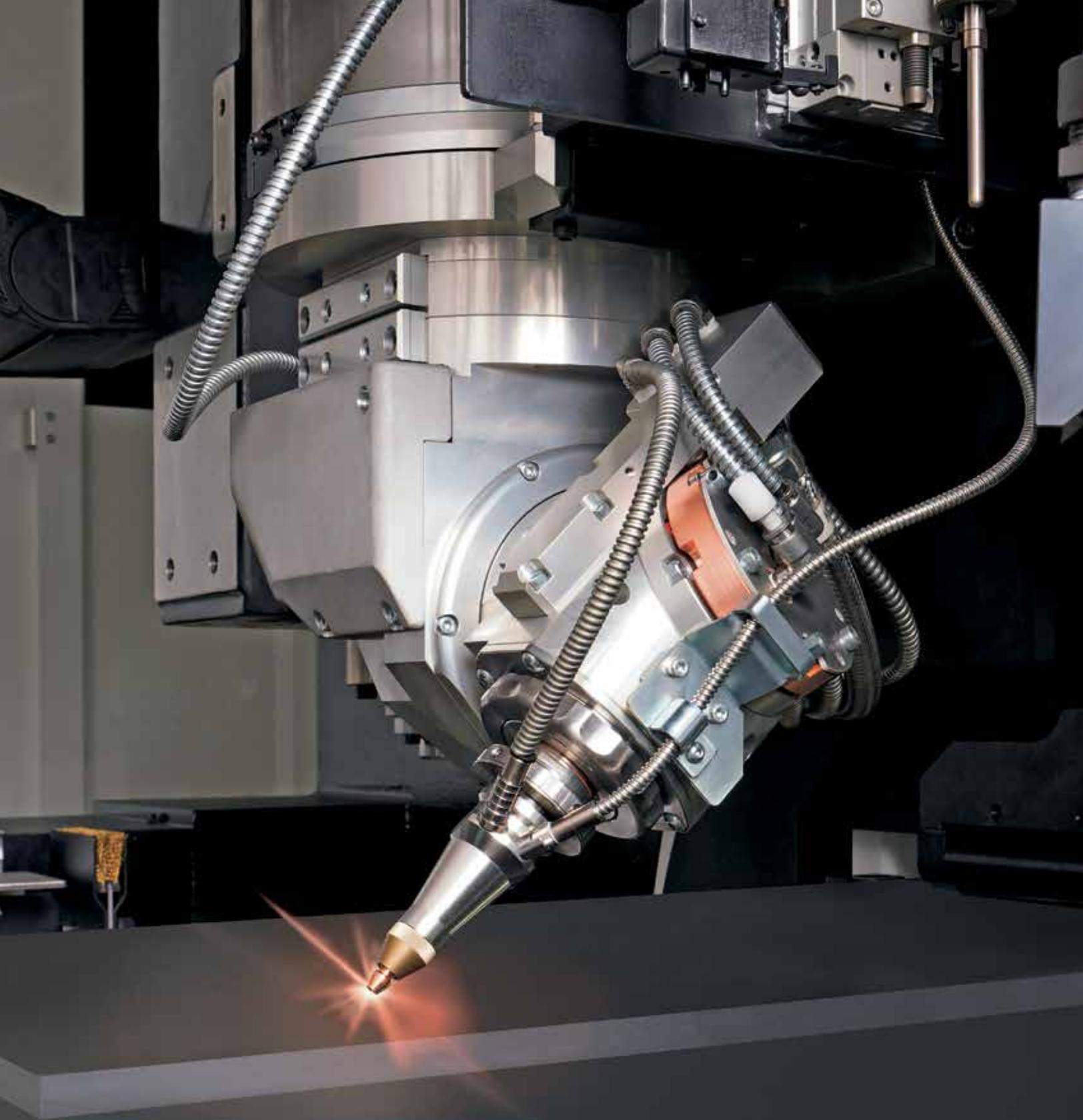
*FG-400 NEO tube-cutting machines offer multi-axis capabilities and beam shaping that enable users to cut a much wider range of structural material not possible on 2D configurations.*
