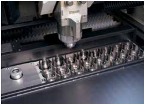
Auto Focus Calibration eliminates the need to have the operator measure, adjust, and set the focal distance by automating the process.
