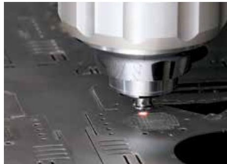
Flash Cut strategies synchronize turning the laser ON / OFF with axis movement to increase throughput.
