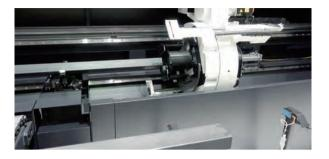
Automatically measures material length after loading onto the machine. This process eliminates manual measuring for each piece of material.
