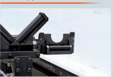
Fixed supports, located beside the V-shaped supports, prevent sagging in longer, small diameter material.
