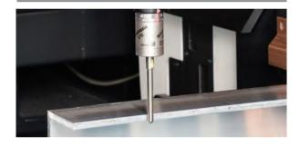
Measures the outer dimension of pipe/structural material and automatically compensates for material distortion to ensure high precision positioning.
