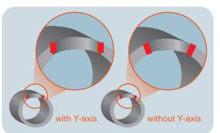
• Bevel cutting with the B-axis provides tight-joint pipes
