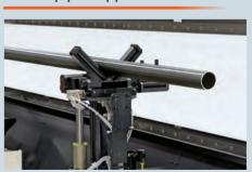
Round material is supported by V-shaped supports. This prevents the material from sagging due to its own weight.
