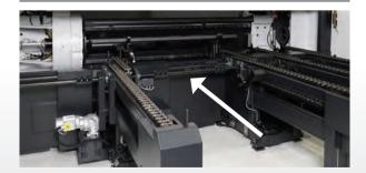
Short materials, which cannot be loaded from the loader side, can be loaded from the unloader side, maximizing material usage.
