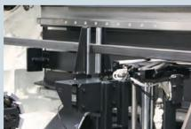
Horizontal workpiece centering for long beams and small pipes by roller prevents material displacement.
