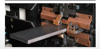
By attaching a jaw dedicated for flat bar cutting, flat bars can be processed.
