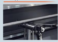
A flat roller controlled by CNC adjusts automatically to support the material and prevent sagging.
