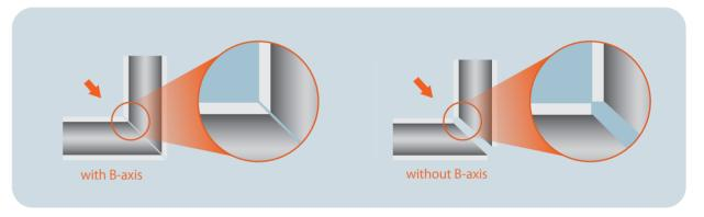
Angled processing with 3D laser head
