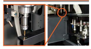
Complete all cutting processes from 3D cutting to tapping in the same machine. The hole to be tapped is cut by the laser and tapped for shorter production lead time and higher productivity. Maximum tapping capability: M16 (5/8 UNC and UNF).
